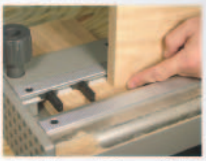
above Set the wood to the correct depth and clamp tight
