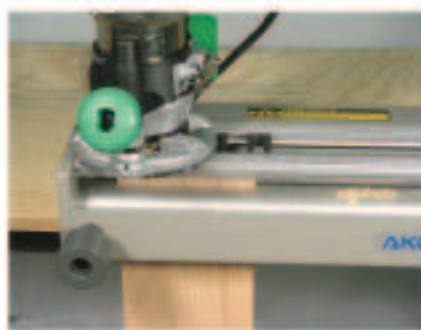
above The router moves easily on the jig to make the cut
