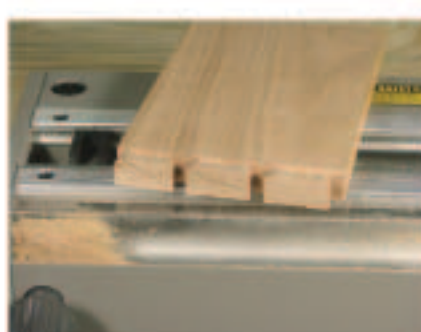
above Careful routing produces the tails
