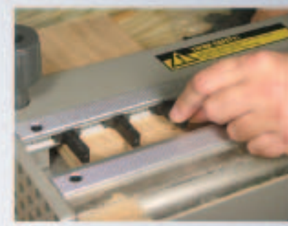
above Install the pin guides on the pencil marks
